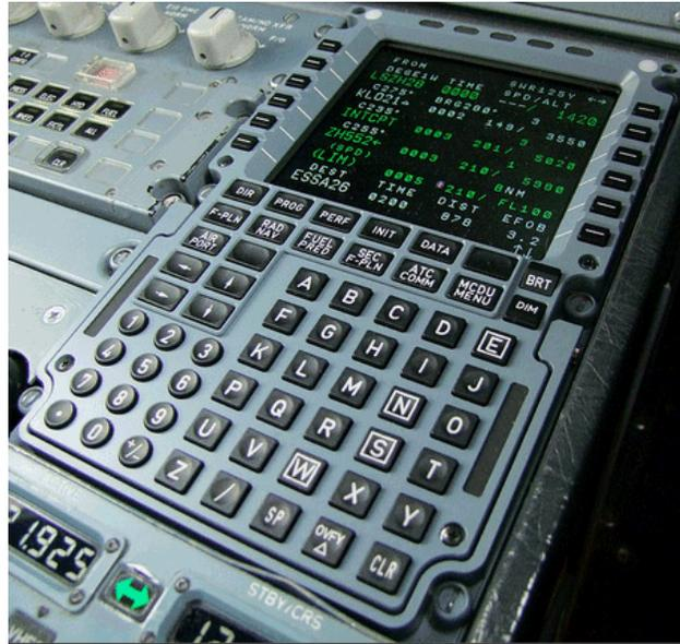
A primary function is in-flight management of the flight plan. Using various sensors (such as GPS and INS often backed up by radio navigation) to determine the aircraft's position, the FMC can guide the aircraft along the flight plan. From the cockpit, the FMC is normally controlled through a Control Display Unit (CDU) which incorporates a small screen and keyboard or touchscreen. The FMC sends the flight plan for display on the EFIS, Navigation Display (ND) or Multifunction Display (MFD).
